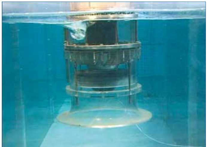
Fig. 59: Laboratory photo of a surface vortex type 3
