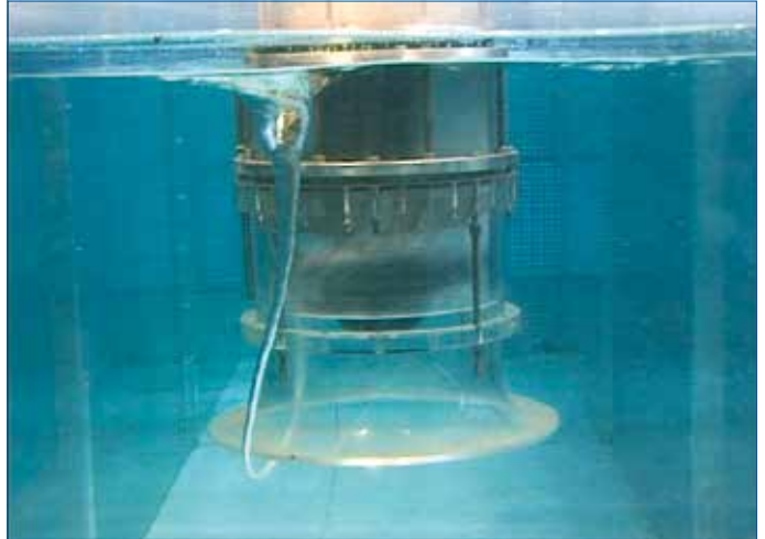
Fig. 58: Laboratory photo of a surface vortex type 6
